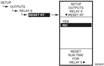
Fig. 49. Setup - Outputs - Relay - Reset Runtime.
