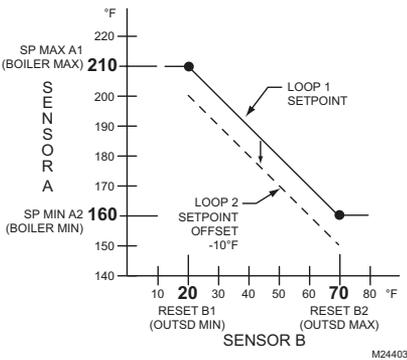
Fig. 71. Reset Curve with Offset for Loop 2.
