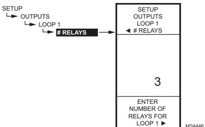
Fig. 38. Setup - Outputs - Loop 1 - Number of Relays.
