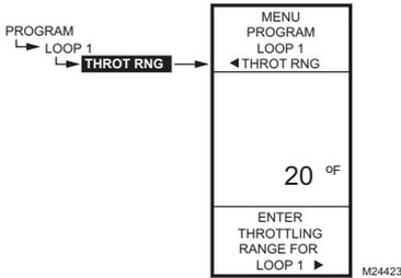
Fig. 55. Program - Throttling Range or Differential.
