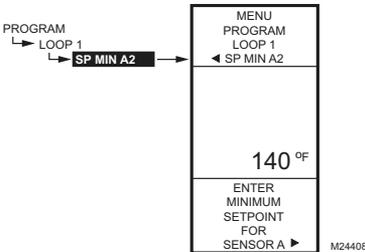
Fig. 65. Program - Sensor A Min. Setpoint.
