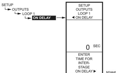
Fig. 41. Setup - Outputs - Loop 1 - On Delay.
