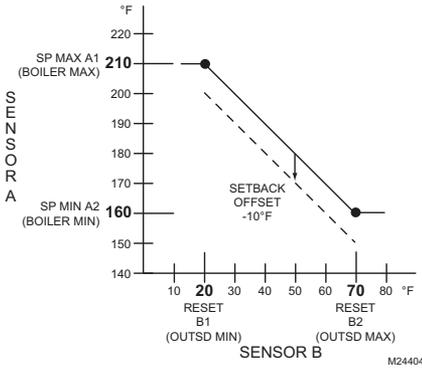
Fig. 60. Reset Curve for Loop 1 with Setback Offset.
