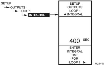
Fig. 39. Setup - Outputs - Loop 1 - Integral.
