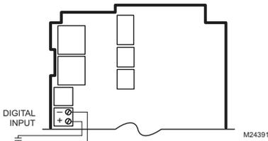
Fig. 12. Wiring for Digital Input (dry contact).
