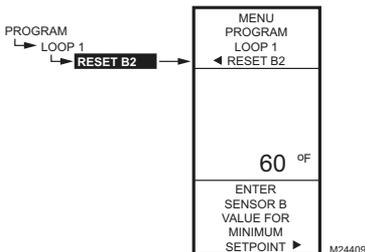
Fig. 66. Program - Sensor B Min. Setpoint.
