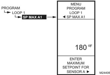
Fig. 63. Program - Sensor A Max. Setpoint.
