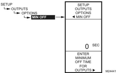
Fig. 33. Setup - Outputs - Options - Min Off Time.
